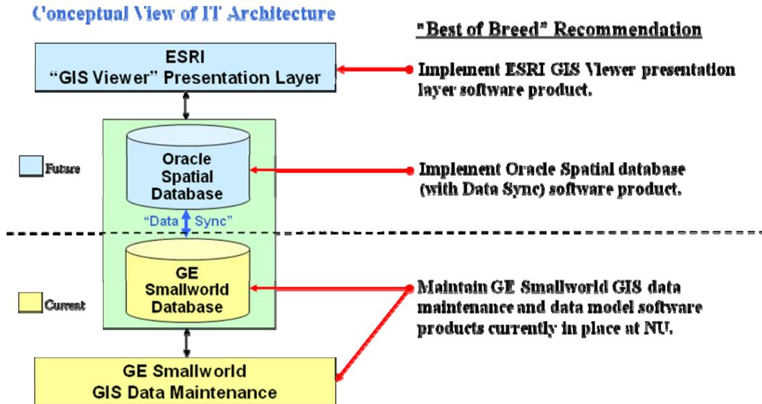
Figure 3: Northeast Utilities Enterprise GIS Architecture
