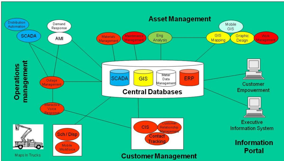
Figure 1: Systems of the Smart Grid
