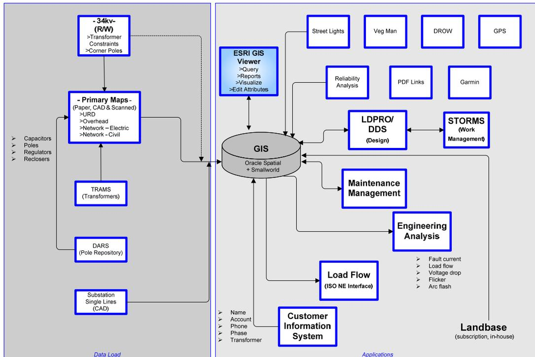
Figure 2: Planned Functional Architecture
